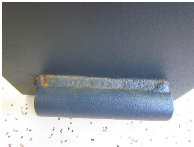
Figure 2. Sample No. 18 appearance after 240 hours in the salt chamber. The degree of rust is marked with 0 in the pipe (more than 50% of total surface corroded), and 6 at the welded zone.
