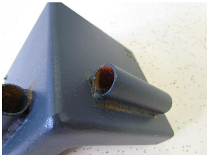
Figure 2. Sample No. 18 appearance after 240 hours in the salt chamber. The degree of rust is marked with 0 in the pipe (more than 50% of total surface corroded), and 6 at the welded zone.
