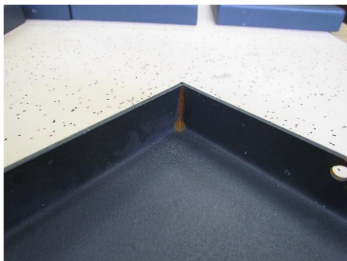
Figure 3. Sample No. 6 appearance after 264 hours in the salt chamber. The degree of rust is evaluated with 9, both in the sharp corners and at the edges.
