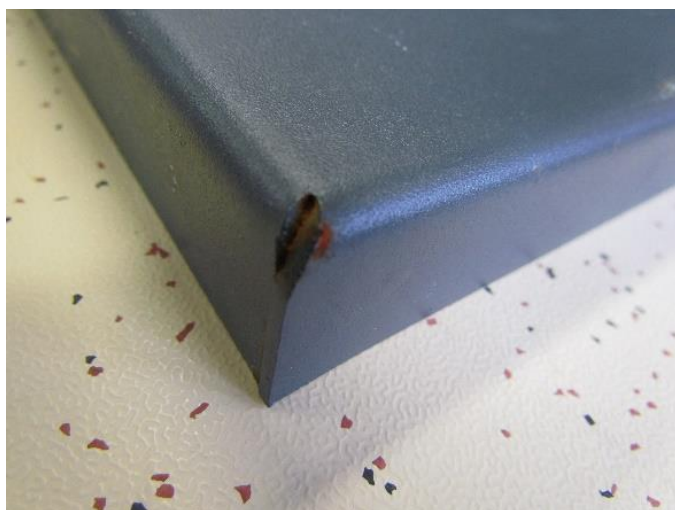
Figure 3. Sample No. 6 appearance after 264 hours in the salt chamber. The degree of rust is evaluated with 9, both in the sharp corners and at the edges.
