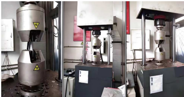
图 3 单轴疲劳与拉伸加载试验机 Figure 3 Uniaxial fatigue and tensile loading testing machine.
