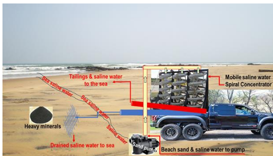
Figure 10 Proposed flow sheet to recover total heavy minerals using sea water with a mobile spiral concentrator along the coastline
