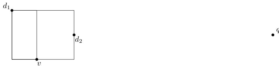
(b) The bounding boxes of the split tree of the point set \{v, d_1, d_2, q\} (except the one of the root of the split tree).
