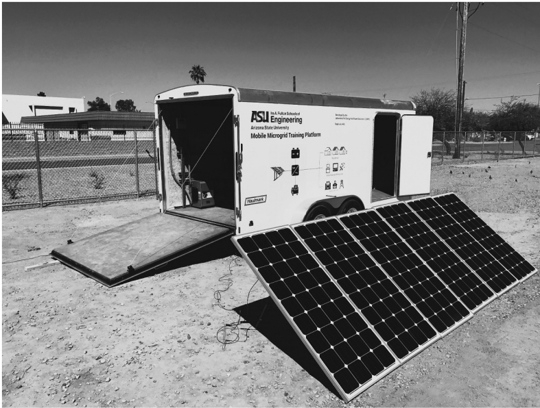
Figure 6. Mobile microgrid training platform.
