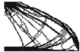
Fig. 9 Results for compliance minimization using a SIREN neural network. No density filter is applied, and all other settings are kept fixed except for the frequency parameter \omega_0 . As \omega_0 increases, high-frequency oscillations emerge in the density field, leading to checkerboard-like patterns
